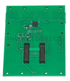
64 pixels (64 low energy + 64 high energy) 1.5 mm pitch, two energies scintillators: GOS - ceramics - high energy, CsI:TI - low energy
