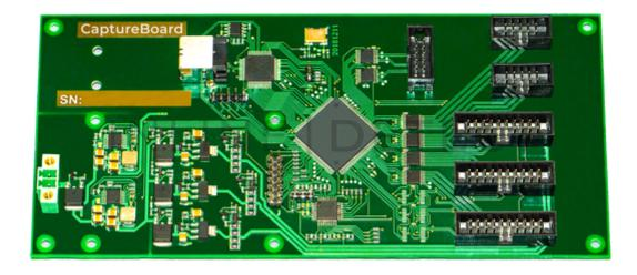
Combines the ionising radiation detectors (LSe-64-1.5 or LDe-64-1.5) and inputs the X-ray image to a computer via USB 2.0 in real time.
