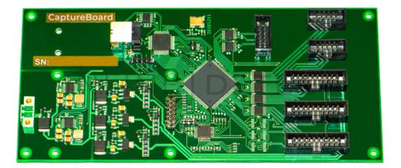
Combines the ionising radiation detectors (LSe-64ru-1.5 or LDe-64-1.5) and inputs the X-ray image to a computer via USB 2.0 or Ethernet in real time.
