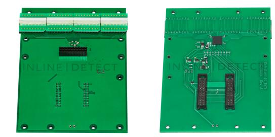
64 pixels (64 low energy + 64 high energy) 1.5 mm pitch, two energies scintillators: GOS - ceramics - high energy, CsI:TI - low energy
